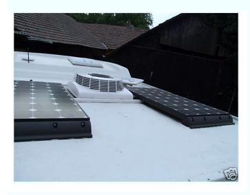
Used with the corner mount sets these spoiler mounts will provide the additional support required for the long sides of larger solar panels.
